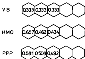
Fig. 1. Three benzene characters, \bar{b}_L (VB), \bar{r}_L^H (HMO) and \bar{r}_L^P (PPP), of pentacene ( L_5 ).
